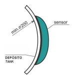
The sensor can adapt to curved surfaces that have a minimum radius of 200 mm.  $\,$
