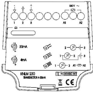
The sensor is factory preset for a reading of 4-20 mA between the margins (D). If you want to calibrate again, connect it as shown in the diagram. Place the float on the bottom and set 4 mA in the instrument by the multiturn potentiometer [4mA]. Do the same with the potentiometer [20mA] placing the float on top.
