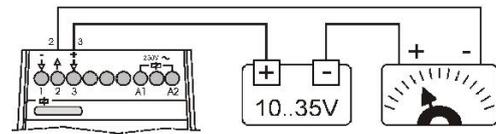
**3 wires:** Connect them to terminals 1, 2 and 3 taking into account the polarity. A voltage source is required for supplying voltage to the current loop.
